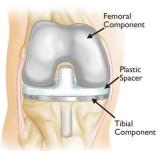
sitting on the bone and a plastic insert, which sits between the metal base on the tibial and femoral component.
